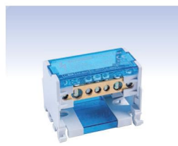
◀ FJ-207/125BE 500V Current: 125A In: 35mm 2 x1(2~3Nm) Out: 25mm 2 x1(2~3Nm) Out: 6mm 2 x5(2~3N.m) 696.000 Rls
