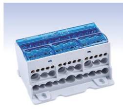
◀ FJ125A-3P 690V Current: 125A In: 35mm 2 x4(8.5Nm) Out: 16mm 2 x12(2.7Nm) Out: 6mm 2 x19(1.2N.m) 2.896.000 Rls
