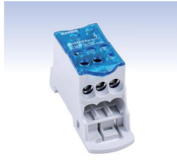
◀ FJ125A 1000V Current: 125A In: 35mm 2 x1(8.5Nm) Out: 16mm 2 x6(3.5Nm) Out: 16mm 2 x1(3.5N.m) 1.137.000 Rls
