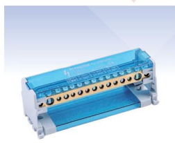
◀ FJ-215/100B 500V Current: 100A In: 25mm 2 x2(2~3Nm) Out: 4mm 2 x6(1.2~1.5Nm) Out: 6mm 2 x7(2~3N.m) 1.345.000 Rls
