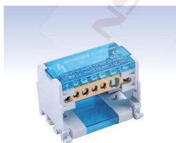
◀ FJ-207/100B 500V Current: 100A In: 25mm 2 x1(2~3Nm) Out: 4mm 2 x3(1.2~1.5Nm) Out: 6mm 2 x3(2~3N.m) 696.000 Rls
