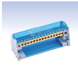
◀ FJ-217/40B 500V Current: 40A In: 16mm 2 x2(2~3Nm) Out: 4mm 2 x15(1.2~1.5Nm) 1.507.000 Rls
