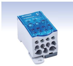
◀ FJ500A 1000V Current: 500A In: 8x24x1mm Out: 35mm 2 x2(4.4Nm) Out: 16mm 2 x5(2.7N.m) Out: 10mm 2 x4(2.7N.m) 3.733.000 Rls
