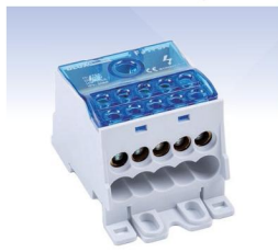
◀ FJ175A 690V Current: 175A In: 70mm 2 x1(5Nm) Out: 16mm 2 x10(3N.m) 2.295.000 Rls
