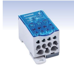
◀ FJ400A 1000V Current: 400A In: 185mm 2 x1(25Nm) Out: 35mm 2 x2(4.4Nm) Out: 16mm 2 x5(2.7N.m) Out: 10mm 2 x4(2.7N.m) 3.501.000 Rls
