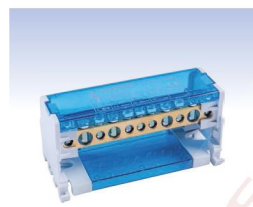
◀ FJ-211/125BE 500V Current: 125A In: 35mm 2 x2(2~3Nm) Out: 25mm 2 x2(2~3Nm) Out: 6mm 2 x7(2~3N.m) 1.021.000 Rls
