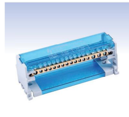
◀ FJ-218/80B 500V Current: 80A In: 6mm 2 x6(2Nm) Out: 4mm 2 x12(1.2Nm) 1.047.000 Rls
