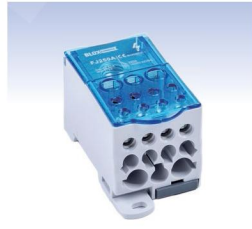
◀ FJ250A 1000V Current: 250A In: 120mm 2 x1(19Nm) Out: 35mm 2 x2(4.4Nm) Out: 16mm 2 x5(2.7N.m) Out: 10mm 2 x4(2.7N.m) 3.291.000 Rls
