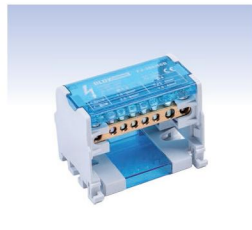
◀ FJ-208/80B 500V Current: 80A In: 6mm 2 x3(2Nm) Out: 4mm 2 x5(1.2Nm) 605.000 Rls
